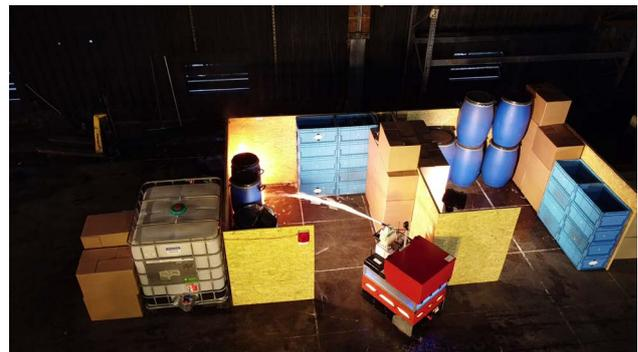
**Figure 7** Experimental test setup for autonomous fire extinguishing
