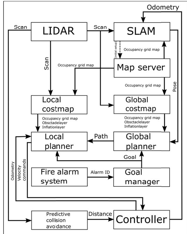
**Figure 4** Overview diagram of the implemented navigation stack
