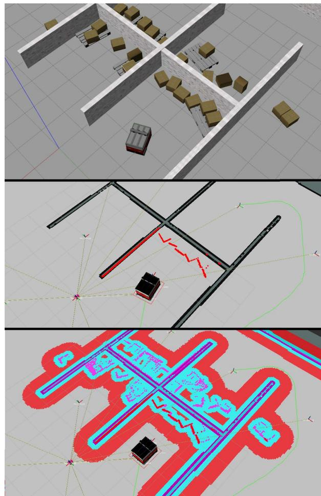
**Figure 5** Simulated environment (top), occupancy grid map (center) and global costmap (bottom)
