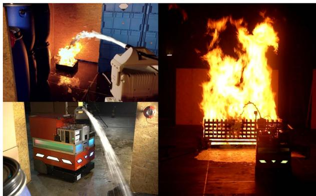
**Figure 8** The developed robot platform during autonomy tests (left) and evaluation of extinguishing capacity similar to DIN EN 3-7 (right)
