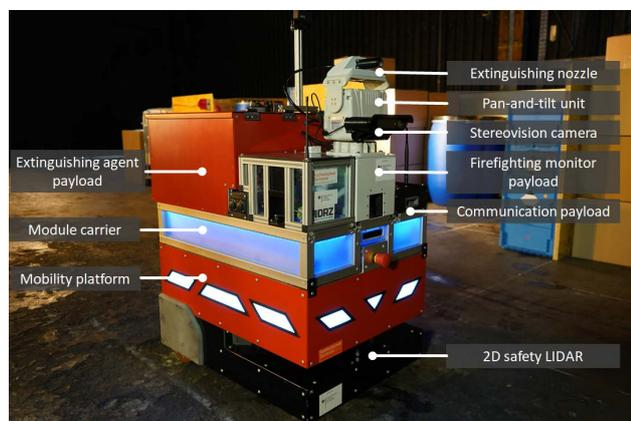
**Figure 2** Mobile robot equipped with an extinguishing agent payload, a firefighting monitor payload and a communication payload.
