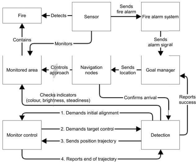
**Figure 3** Concept of an autonomous firefighting operation
