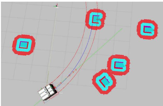
**Figure 6** Predictive Collision Avoidance (PCA). Predicted search area (red) and minimal distance to possible collision (blue)
