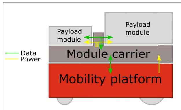
**Figure 1** Schematic representation of the modularisation concept
