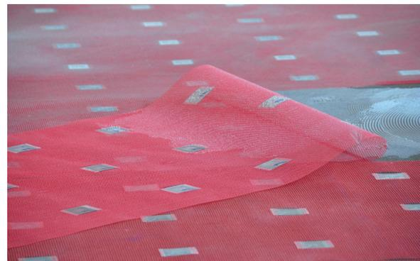
**Figure 1** Underlay with integrated RFID tags for localization of mobile robots
