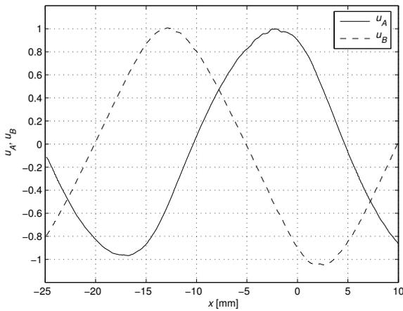
Fig. 3. Optimal current commands for constant force
