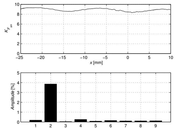
Fig. 1. Force function  $K_F(x)$  with spectrum
