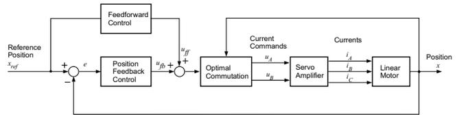
Fig. 5. Controller design
