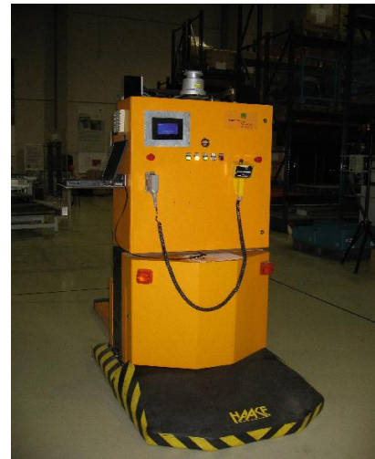
Fig. 4. Forklift Truck with Wireless Sensor Network
