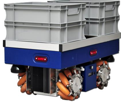
Figure 5. Omnidirectional vehicle with Mecanum wheels
