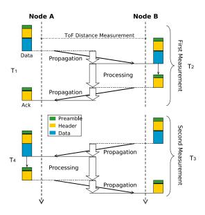
Fig. 2. Symmetrical Double-Sided Two Way Ranging [18]
