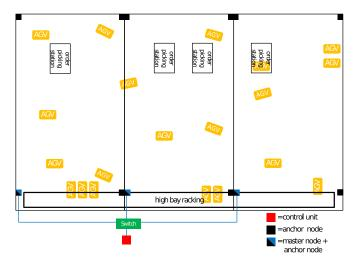
Fig. 3. Wireless network with three cells and router
