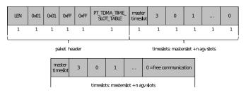
Fig. 4. Time slot table and superframe design
