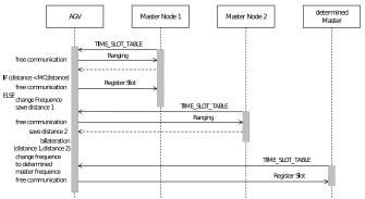
Fig. 7. Initialisation and cell assignment
