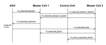
Fig. 6. Sequence chart of handover procedure
