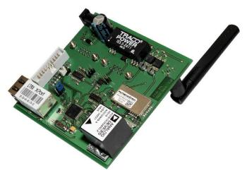
Fig. 8. Wireless sensor node for anchors and mobile tags
