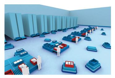
Fig. 1. Swarm of mobile robots in a distribution center © Fraunhofer IML
