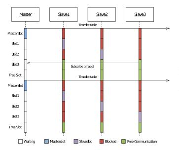
Fig. 5. Allocation of time slot
